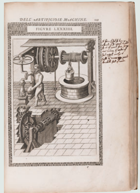
Figure 9: Geared mechanism for lifting well water, engraving from The Diverse and Complex Machines , a 1588 work by Agostino Ramelli annotated with handwritten commentary by Thomas Arundell. Elizabethan Club Endowment Fund (1911), Elizabethan Club.
